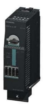
F-DS1E-X FOR ET 200S FAILSAFE DIRECT STARTER SETTING RANGE 2.4...8A, MECHANICAL SWITCHING ELECTRONIC PROTECTION AC-3, TO 3KW/400V, CAN BE EXPANDED FOR BRAKE CONTROL MODULE FOR 2DI CONTROL MODUL
