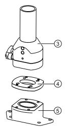
4. Screw on the basic adapter (5) from below to the intermediate plate (4): To do so insert the four screws M6 x 12 from the accessories kit of the adapter set through the upper holes of the basic adapter and fasten the screws into the inner treaded holes of the intermediate plate. Check that the seal is properly seated.
