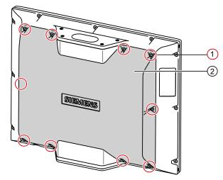
2. Remove the rear wall of the housing ② and store it in a secure location.
