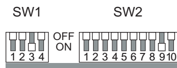
Figure 6-33 Default settings of the DIL switches SW1 and SW2
