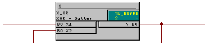
Figure 5-43 Example of a Feedback from the Output to the Input of a Function Module
