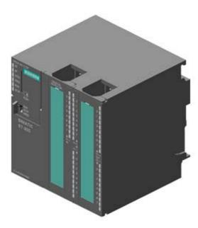
\*\*\* SPARE PART\*\*\* SIMATIC S7-300, CPU 314C-2DP COMPACT CPU WITH MPI, 24 DI/16 DO, 4AI, 2AO, 1 PT100, 4 FAST COUNTERS (60 KHZ), INTEGRATED DP INTERFACE, INTEGRATED 24V DC POWER SUPPLY, 96 KBYTE WORKING MEMORY, FRONT CONNECTOR (2 X 40PIN) AND MICRO MEMORY CARD REQUIRED
