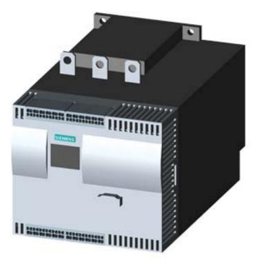
SIRIUS soft starter Values at 400 V, 40 °C Standard: 134 A, 75 kW Inside-delta: 232 A, 132 kW 200-460 V AC, 230 V AC spring-type terminals
