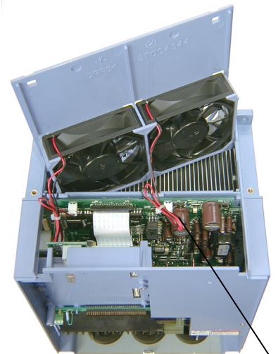
PWB connector for fan assembly wiring
