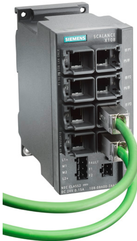
Figure 5-2 Plugging in the IE FC RJ45 Plug 180
