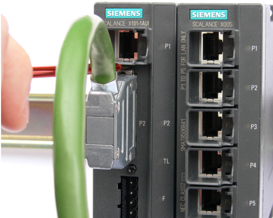
Figure 5-4 Locking or unlocking the D-sub connector
