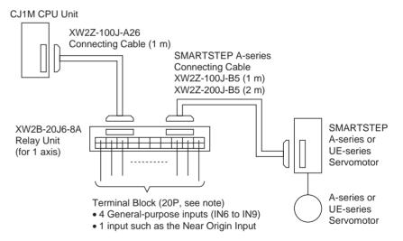
**Note** When using a One-axis Relay Unit (connected to pulse output 0), general-purpose outputs 2 and 3 (OUT2 and OUT3) and PWM(891) output 1 (OUT5) cannot be used.
