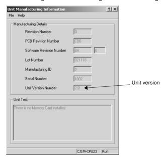
Use the above display to confirm the unit version of the CPU Unit connected online.
