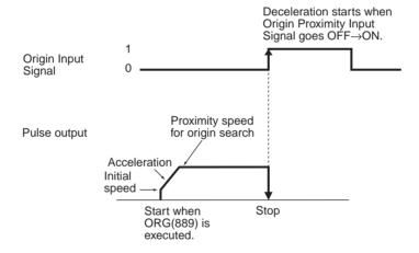
Origin Search Operating Mode and Origin Detection Method Settings The following examples explain how the operation patterns are affected by the origin search operation and origin detection method settings.
