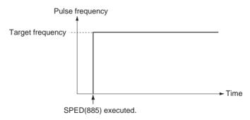
In independent mode, pulse output will stop automatically when the number of pulses set with PULS(886) in advance have been output. In continuous mode, pulse output will continue until stopped from the program.
