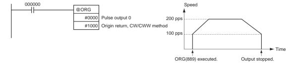
The PLC Setup parameters are as follows:
