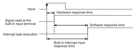
Built-in interrupt input response time = Hardware interrupt response time + Software interrupt response time
