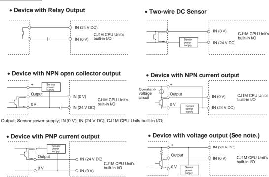
Note Do not use the following wiring with voltage-output devices.
