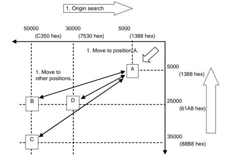
Note The X and Y axes are moved independently, i.e., interpolation is not performed.
