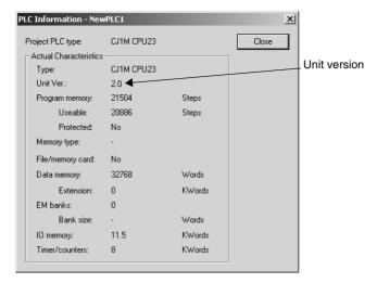
Use the above display to confirm the unit version of the CPU Unit.
