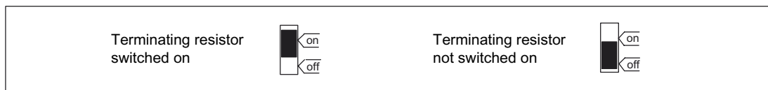
Figure 6-4 Terminating resistor switched on and off
