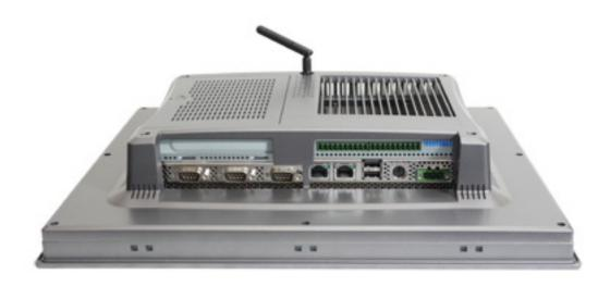
Figure 1.2 TPC-1571H - I/O Port Arrangement (Antenna is optional. Use P/N:1750000318 to order)
