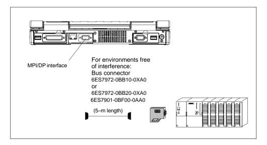
Fig. 3-12 Connection Using the MPI/DP Interface
