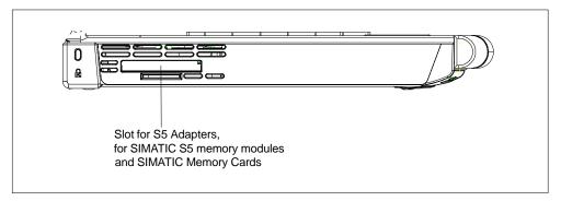
Fig. 3-7 S5 Module Programming Interface
