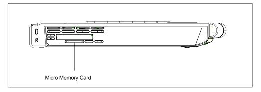
Fig. 3-9 Slot for Micro Memory-Cards
