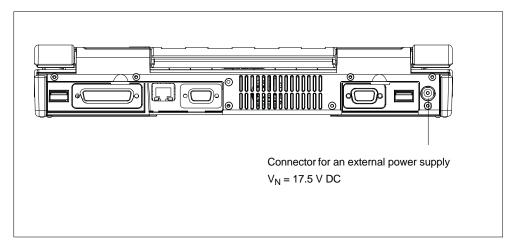
Fig. 3-2 Power supply connection
