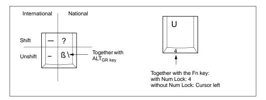
Fig. 2-1 The Keyboard Labeling System
