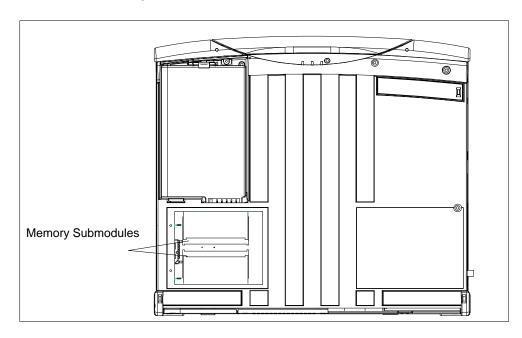
Fig. 4-1 Positions of the SO DIMM Memory Submodules
