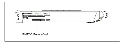
Fig. 3-8 Slot for SIMATIC Memory Cards
