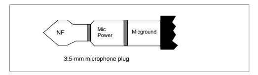
Fig. 3-5 Pin assignment of the microphone plug
