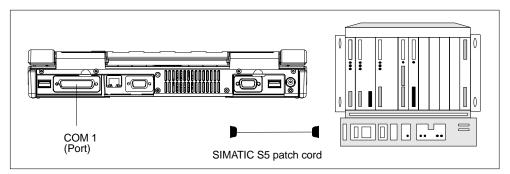
Fig. 3-11 Connecting to an S5 PLC
