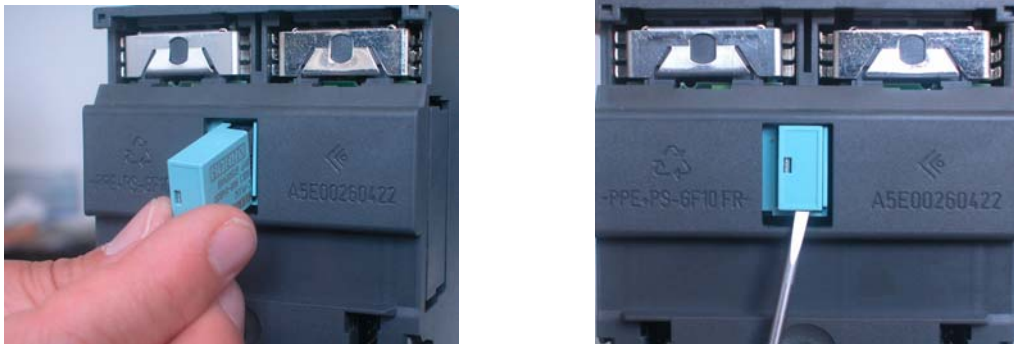
Figure 3-2 Fitting the C-PLUG and removing it from the CP with a screwdriver
