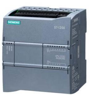
\*\*\*SPARE PART\*\*\* SIPLUS S7-1200 CPU 1212C DC/DC/DC -25 ... +70 DGR C MIT CONFORMAL COATING BASED ON 6ES7212-1AD30-0XB0 . COMPACT CPU, DC/DC/DC, ONBOARD I/O: 8 DI 24V DC 6 DO 24 V DC 2 AI 0 - 10V DC, POWER SUPPLY: 20.4 -28.8 V DC PROGRAM/DATA MEMORY: 25 KB
