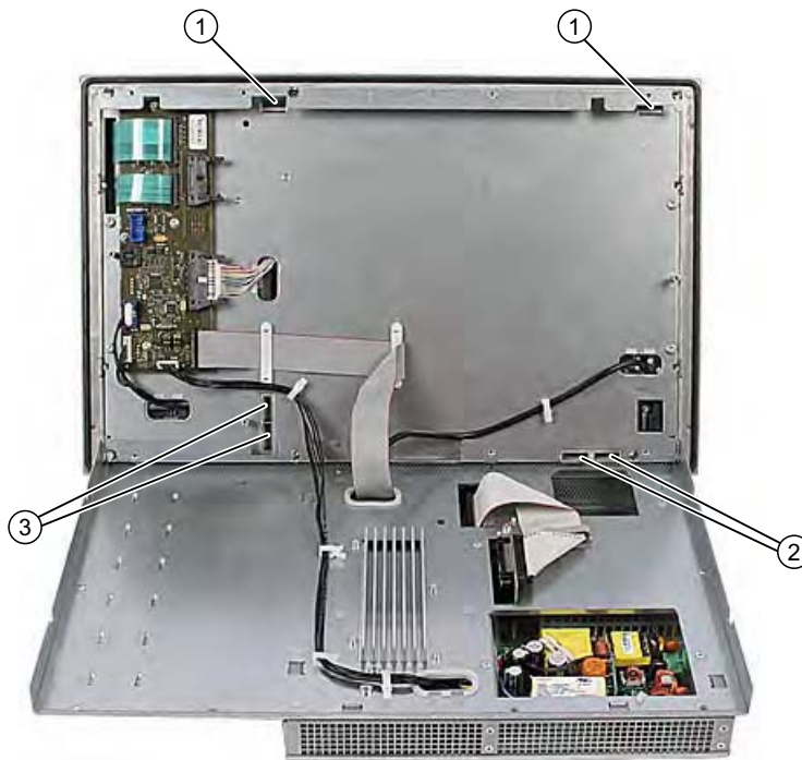
Figure 4-3 Device rear with connections and slots for the labeling strips
