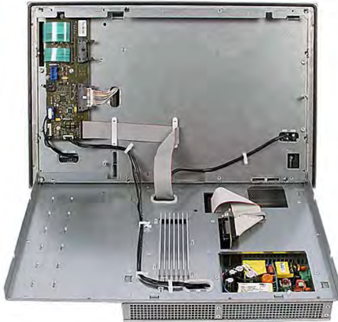
Figure 4-2 Example 12" touch screen device: Separating the computer unit from the control unit
